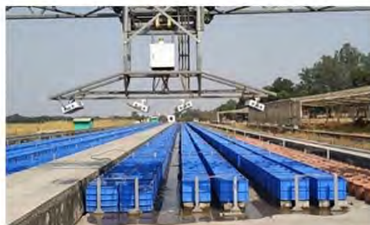
Fig. 1 The LeasyScan 9 high-throughput phenotyping platform used to gather the data. The picture shows the dual position (2 complementary, partially overlapping scanners capture the same area). The mounted scanners are moving over the field to capture the data (~2 500 m 2 area in 90 minutes).
