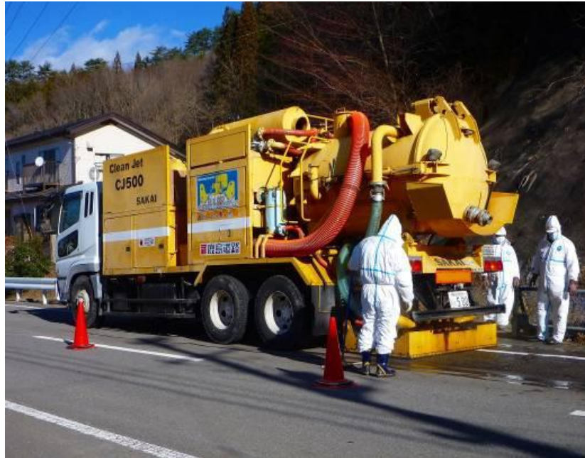
Fig. 19. High-pressure washing of roads using large vehicles (source: Masayuki, 2012: 52)
